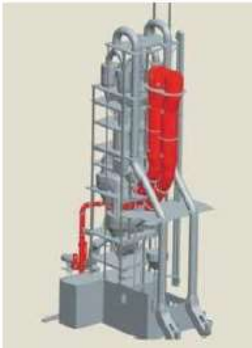
Calciner loop duct
